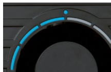
In "Humidifier" mode the LEDs are lit blue
